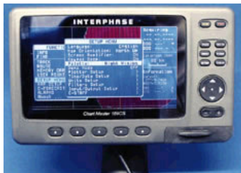
The Chart Master 169CS (pictured) has a separate DGPS receiver, while the 169CSi's receiver is internal. Both models should be easy to use for anyone familiar with personal computers, PDAs or similar menu-driven plotters.
